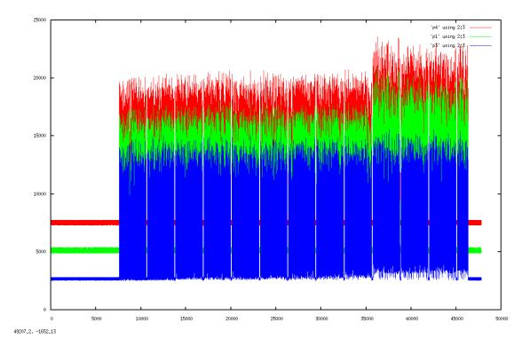
Nodes "p2" and "s1", connected to WRS1, feature a latency of 225-380 microseconds: never less than 225 and never more than 382. As shown in the following figure (this is drawn with dots instead of lines, to avoid red items to be completely overlaid by green items; the two data sets are quite overlapping)
