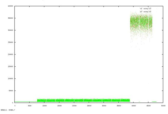
At least 350 of these 380 microseconds are spent in the WRS2-to-WRS1 link and the input queue of the port of the node. Interestingly, the WRS2-to-WRS1 link is completely empty.
