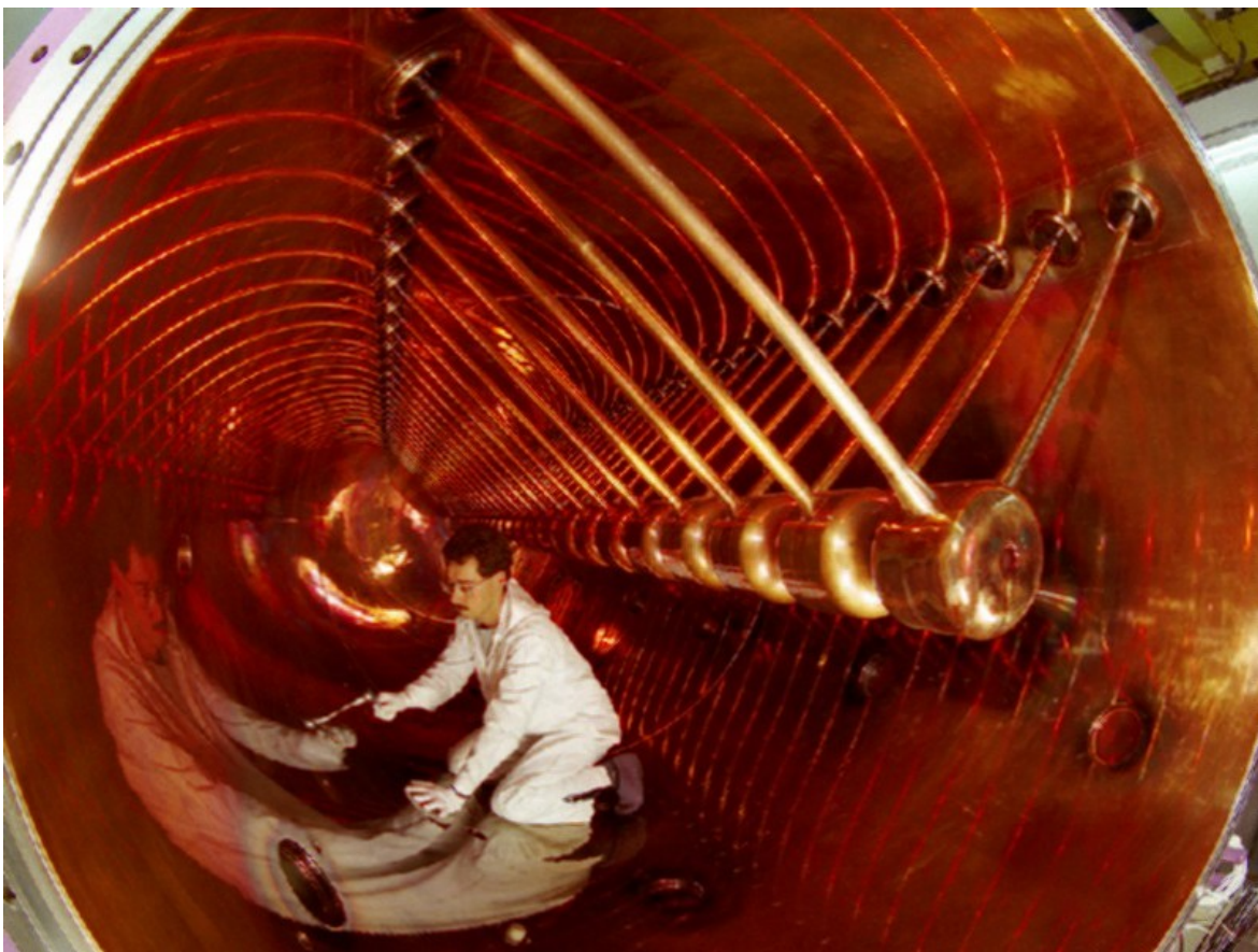
FIGURE 3.2: Inside of an Alvarez tank at GSI. The drift tubes in the centre are supplied with the RF voltage by the diagonal struts. [52]
