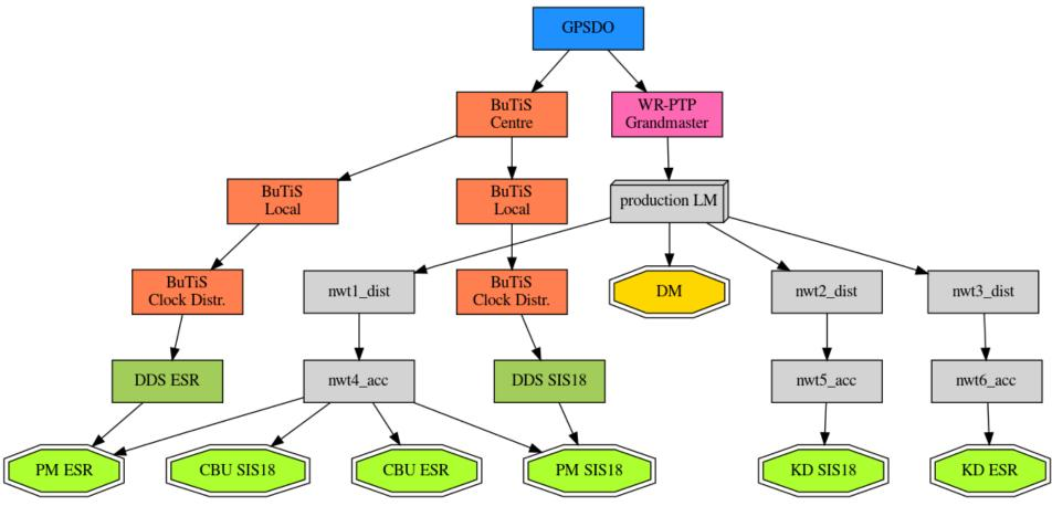
Components: GPSDO (blue), White Rabbit Grandmaster (cyan) and Switches (grey), rf-clock distribution system (BuTiS, brown), rf-group-DDS systems (dark green), nodes of the b2b system (light green) and Data Master of the Machine Timing System (yellow). Nodes with double-lined borders broadcast messages to the White Rabbit network.
