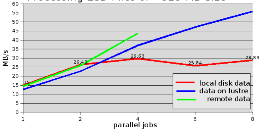
Aggregate Data Throughput for Analysis Jobs Processing ESD Files of ~525 MB Size
