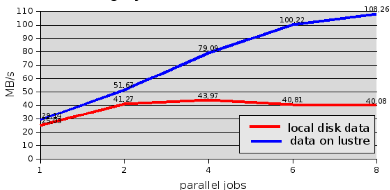
Aggregate Data Throughput for Analysis Jobs Processing Pythia Files of ~529 MB Size
