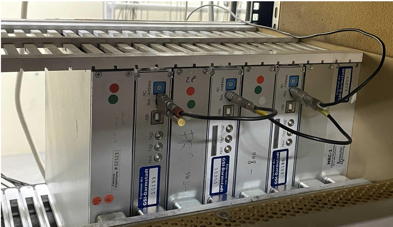
Fig.5 Back side of the NIM crate. Make sure connection between MRC-1 and CFDs is there!
