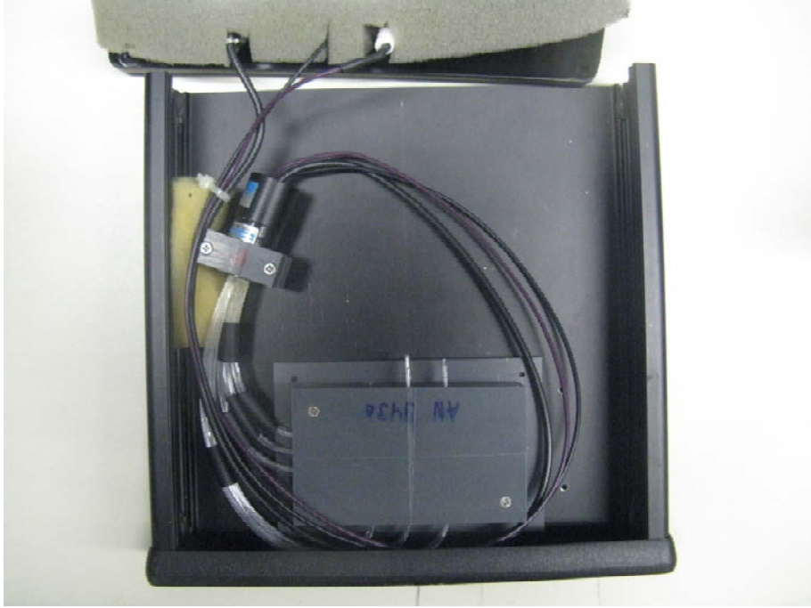
Figure 13: Photo of the opened TPC scintillator mask
