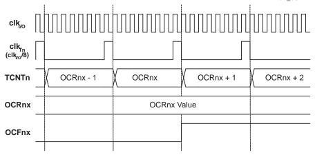
Figure 13-12 shows the count sequence close to TOP in various modes. When using phase and frequency correct PWM mode the OCRnx Register is updated at BOTTOM. The timing diagrams will be the same, but TOP should be replaced by BOTTOM, TOP-1 by BOTTOM+1 and so on. The same renaming applies for modes that set the TOVn flag at BOTTOM.
