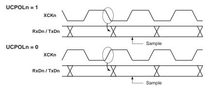
The UCPOLn bit UCRSnC selects which XCKn clock edge is used for data sampling and which is used for data change. As Figure 17-3 shows, when UCPOLn is zero the data will be changed at rising XCKn edge and sampled at falling XCKn edge. If UCPOLn is set, the data will be changed at falling XCKn edge and sampled at rising XCKn edge.
