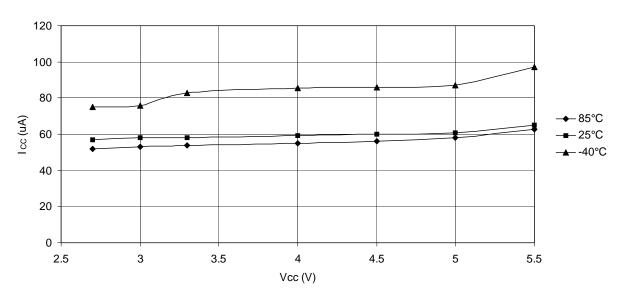
Figure 28-36. Programming Current vs. Operating Voltage
