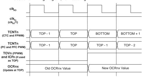
Figure 13-12. Timer/Counter Timing Diagram, no Prescaling
