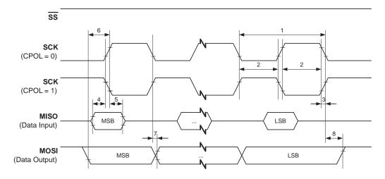
Figure 26-5. SPI Interface Timing Requirements (Slave Mode)
