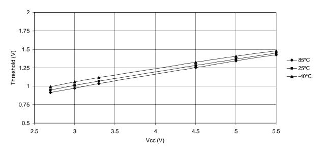
Figure 2. I/O Input Hysteresis vs. Vcc
