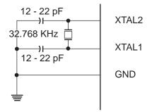
12-22 pF capacitors may be necessary if the parasitic impedance (pads, wires & PCB) is very low.
