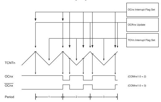
The Timer/Counter Overflow Flag (TOV2) is set each time the counter reaches BOTTOM. The interrupt flag can be used to generate an interrupt each time the counter reaches the BOTTOM value.
