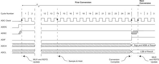
Figure 21-5. ADC Timing Diagram, Single Conversion
