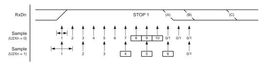
The same majority voting is done to the stop bit as done for the other bits in the frame. If the stop bit is registered to have a logic 0 value, the Frame Error (FEn) flag will be set.
