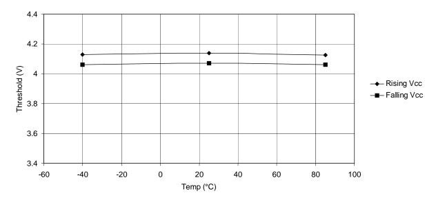
Figure 28-25. BOD Thresholds vs. Temperature (BOD level is 2.7V)
