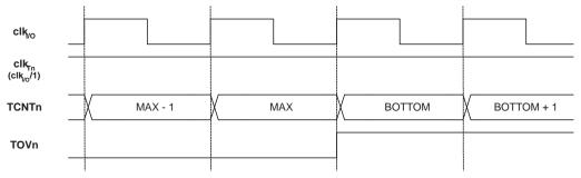
Figure 12-9 shows the same timing data, but with the prescaler enabled.
