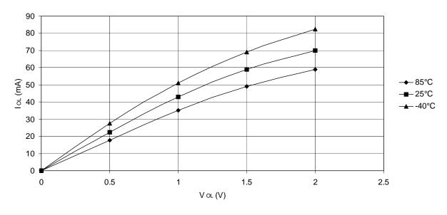
Figure 28-22. I/O Pin Sink Current vs. Output Voltage (Vcc = 2.7V)
