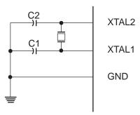
The Oscillator can operate in three different modes, each optimized for a specific frequency range. The operating mode is selected by the fuses CKSEL3..1 as shown in Table 5-3.
