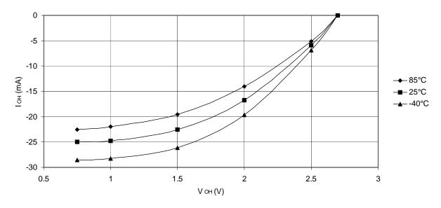
Figure 28-21. I/O Pin Sink Current vs. Output Voltage (Vcc = 5V)
