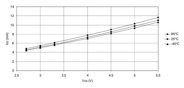
Figure 28-9. Idle Supply Current vs. Vcc (Internal RC Oscillator 1 MHz)
