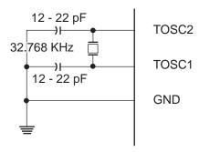
A external clock can also be used using TOSC1 as input. Setting AS2 and EXCLK enables this configuration.
