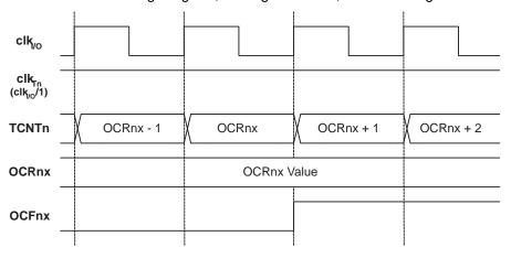
Figure 13-11 shows the same timing data, but with the prescaler enabled.
