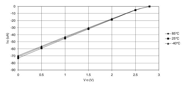
Figure 28-17. Reset Pull-up Resistor Current vs. Reset Pin Voltage (Vcc = 5V)
