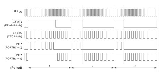
In this example, Timer/Counter0 provides the carrier, while the modulating signal is generated by the Output Compare unit C of the Timer/Counter1.
