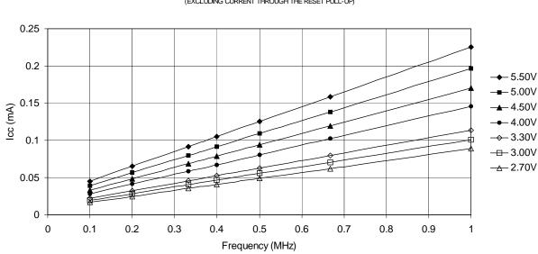
RESET SUPPLY CURRENT vs. FREQUENCY (25°C, 0.1 - 1 MHz) (EXCLUDING CURRENT THROUGH THE RESET PULL-UP)
