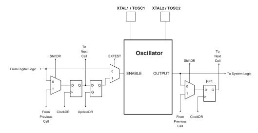
Table 23-5 summaries the scan registers for the external clock pin XTAL1, oscillators with XTAL1/XTAL2 connections as well as external Timer2 clock pin TOSC1 and 32kHz Timer2 Oscillator.
