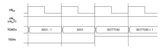
Figure 14-10 shows the same timing data, but with the prescaler enabled.
