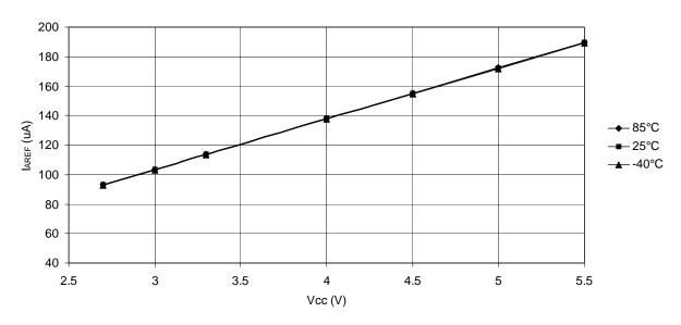
Figure 28-35. Analog Comparator Current vs. Operating Voltage
