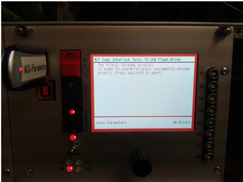
**NOTE!!!:** It is normal that the Interlock text file is already present on the USB stick and there is no problem to overwrite it because it will be the same loaded in the step a above.
