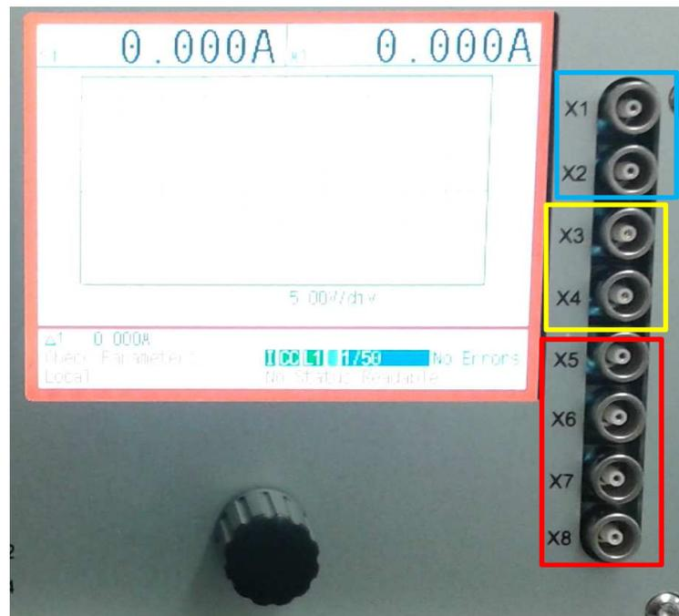
The output values of X1 and X2 are configurable in PCA. On X4 it is connected a square waveform 0/+3.3V with a frequency of 20 KHz generated by a function generator. Let's proceed step by step:
