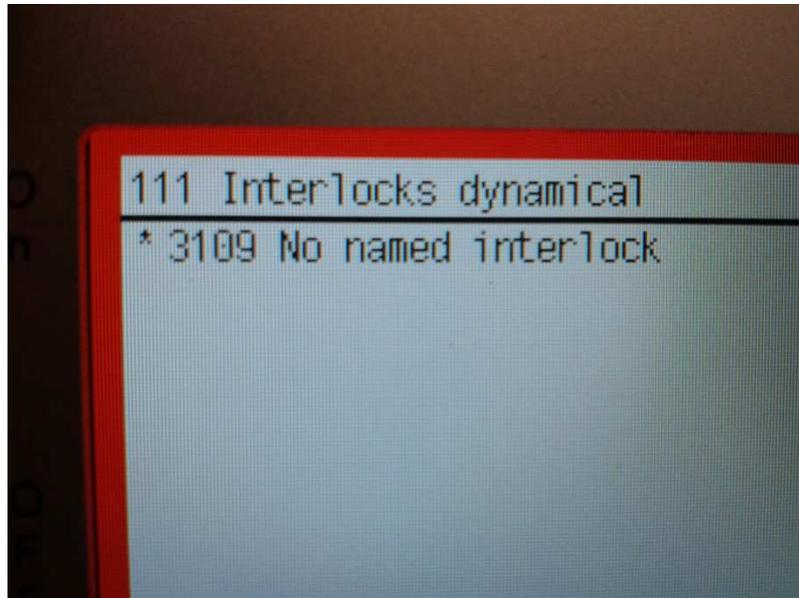
If the **111 Interlocks dynamical** Window is not displayed automatically, in order to check the activated interlock, press the incremental encoder, select first **1 System Overview** then **11 Interlocks** and finally **111 Interlocks dynamicals**.
