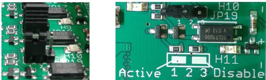
It means that the corresponding interlock is enabled. Without any optical signal in input, the interlock has to be triggered and this is reported by a red LED on just below the jumper. At this point of the test, all the LEDs under the jumpers from JP1 to JP9 have to be on (red).
