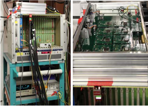
Figure 2: VME crate with hardware setup (left) at GSI beam line. Two prototype boards with 8 CFC-ASICs (right) each were connected with one MWPC.
