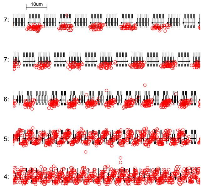
Fig. 6. Overlay of inverter chain test structure layout and position of SET events. The radius of the circle is equivalent to  $3\sigma$  position accuracy or approx. 600 nm.
