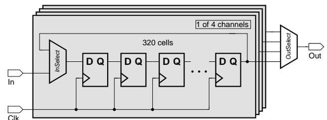
Fig. 2. Block diagram of a flip-flop group for SEU testing. Each group consists out of four channels with different flip-flop implementations.
