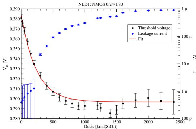
Fig. 7. Threshold voltage shift and leakage current of a single NMOS transistor ( $W/L = 0.24 \mu\text{m}/1.80 \mu\text{m}$ ) for different dose levels.
