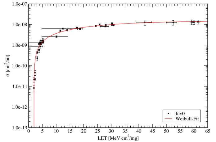
Fig. 4. Weibull fit of the SET cross section of a minimum sized inverter.
