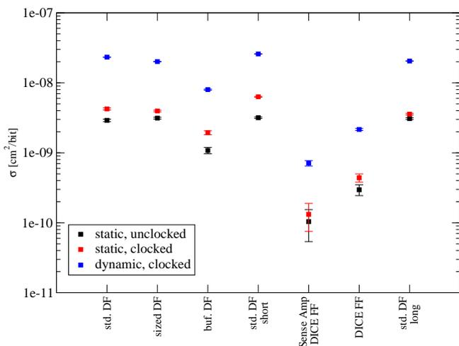
Fig. 5. Saturated SEU cross section of all flip-flop test structures. The applied clock frequency was 100MHz.
