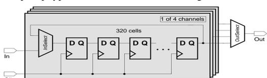
Fig. 2.: Block diagram of a flip-flop group for SEU testing.
