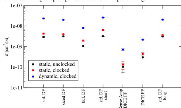
Fig. 5.: Saturated SEU cross section of all flip-flop test structures.
