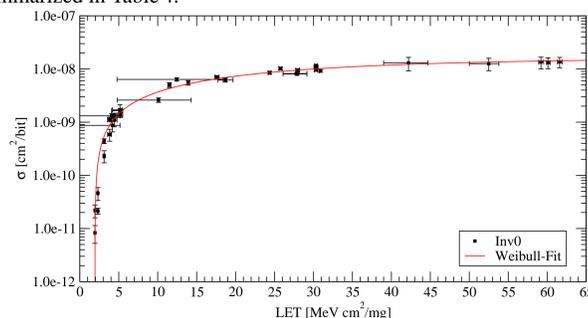
Fig. 4.: Weibull fit of the SET cross section of a minimum sized inverter.
