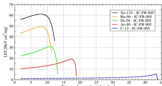
Fig. 3.: LET range for the available ions of the 2008/2009 testing.
