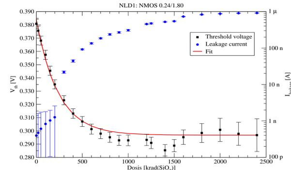
Fig. 7.: Threshold voltage and leakage current of a single transistor for different dose levels.
