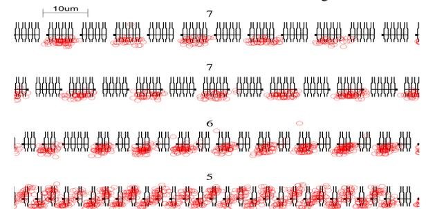
Fig. 6.: Overlay of inverter chain test structure layout and position of SET events. The radius of the circle is approx. 600 nm.
