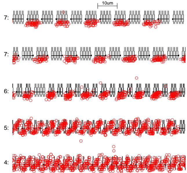
Figure 1: Overlay of inverter chain test structure layout and position of SET events. The radius of the circle is equivalent to  $3\sigma$  position accuracy or approx. 600 nm.
