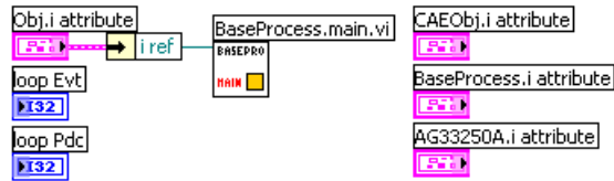
Fig. A.5. Main method of the AG33250A class. It is just a wrapper around the main method of the BaseProcess class.
