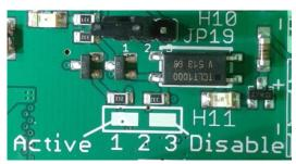
It means that the corresponding interlock is enabled. Without any optical signal in input, the interlock has to be triggered and this is reported by a red LED on just below the jumper. At this point of the test, all the LEDs under the jumpers from JP1 to JP9 have to be on (red).
