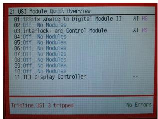
NOTE!: If the ICM module is not reported in the list, please turn the module off and on and try again a USI re-scan (step a above).
