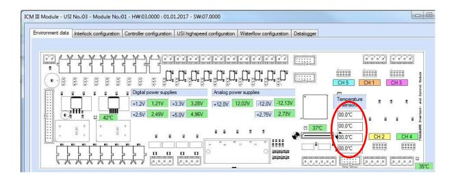
f. Spray some cooling liquid on the external temperature sensor and play with the jumpers on it in order to see the external temperature value on each text box in PCA.
