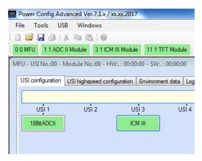
b. In the *Environment data* tab window check if the temperature reported by the three embedded temperature sensors are different from 255 (in red below).
