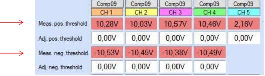
e. Repeat the test also for the negative threshold following the same steps performed in the point d above.
