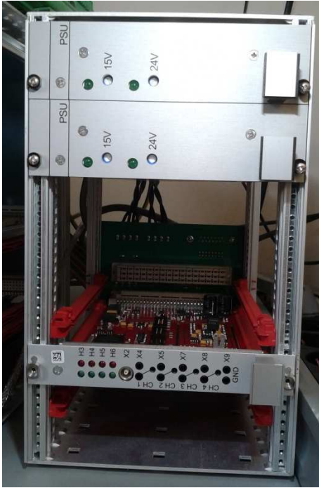
Figure 2-2 Power Supply Shelf
