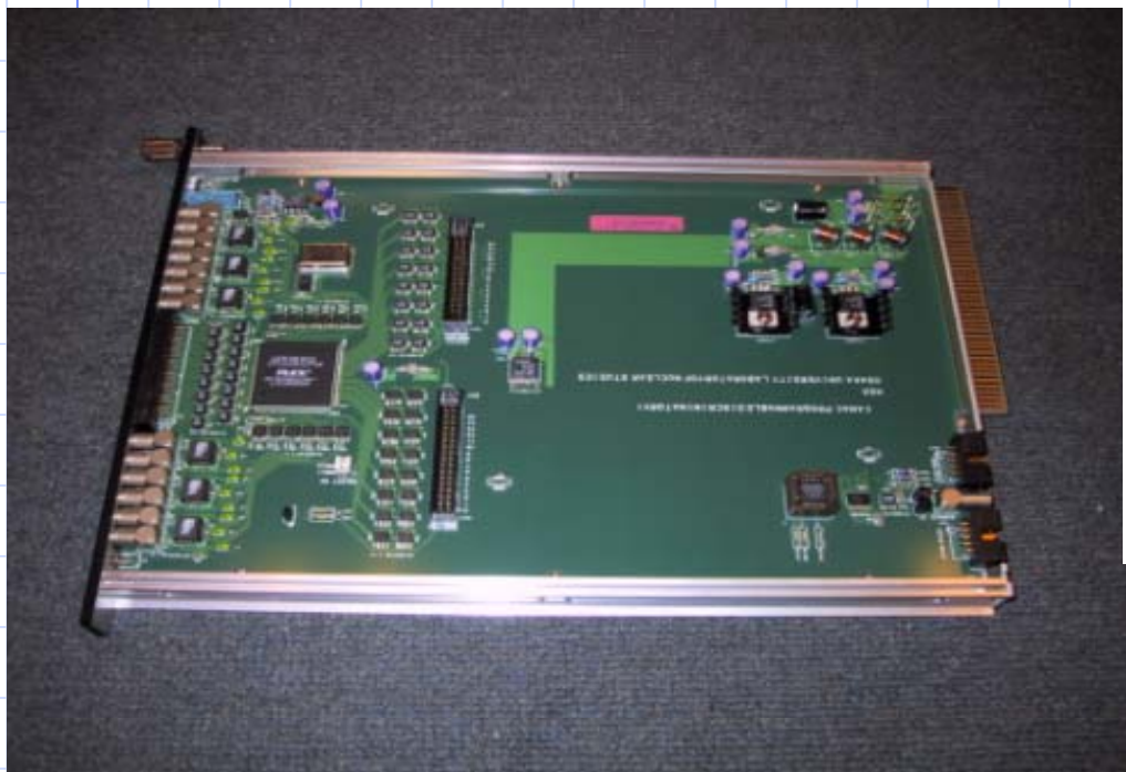
Fig. 2: 12 channel intelligent discriminator.
